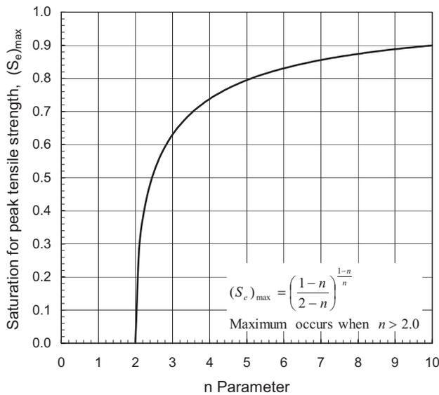
**Fig. 5.** Theoretical functions for (a) the magnitude of the peak tensile strength as a function of the pore size spectrum parameter  $n$ ; (b) the equivalent degree of saturation for the peak strength as a function of the pore size spectrum parameter  $n$
