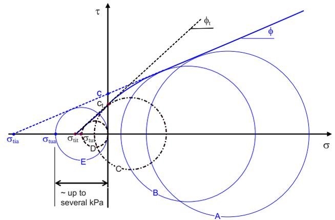
**Fig. 3.** Conceptual illustration of the proposed theory for non-M-C failure of sand in tensile stress regime
