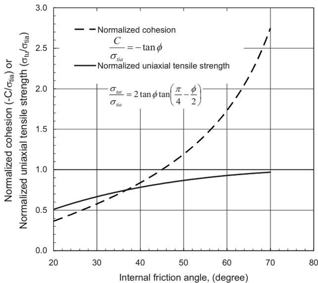
**Fig. 2.** Illustration of the abilities of uniaxial tensile strength and apparent cohesion in mobilizing isotropic tensile stress into shear stress as functions of friction angle
