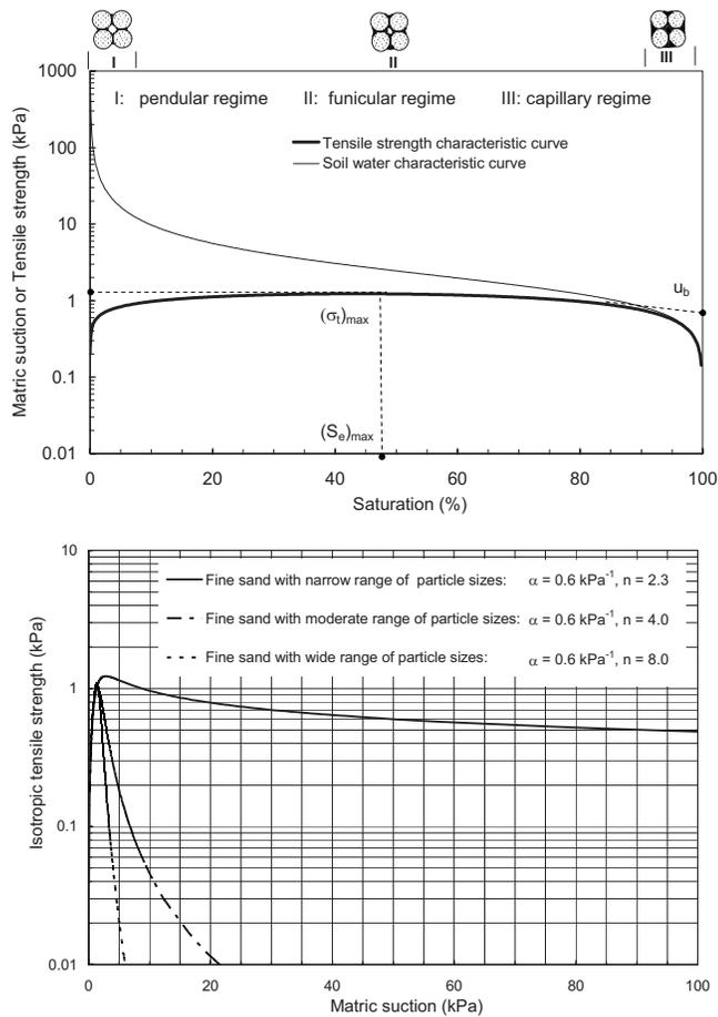
**Fig. 4.** Illustration of the characteristics of tensile strength of sand: (a) interrelationship between soil water retention curve and tensile strength characteristic curve for over the entire saturation range; (b) tensile strength of fine sand as a function of soil suction for different pore size distributions
