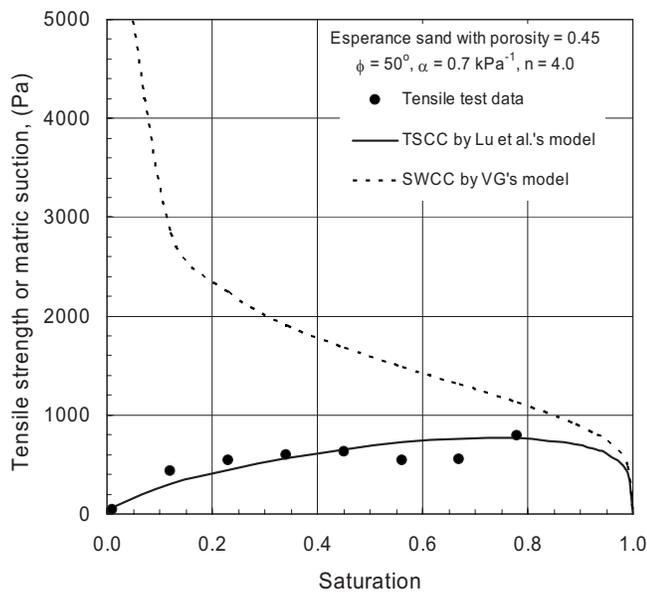
**Fig. 7.** Comparisons of the measured and predicted soil water retention curve, tensile strength characteristic curve for Esperance sand with porosity of (a) 0.4; (b) 0.45
