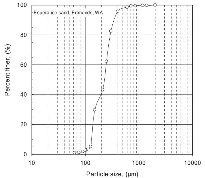
**Fig. 6.** Particle-size distribution for Esperance sand, from Edmonds, Washington
