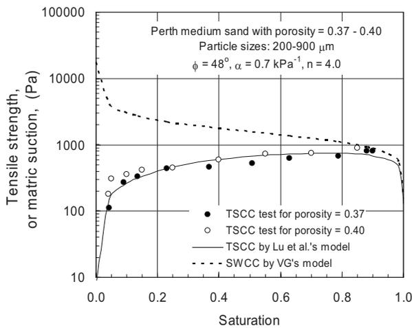
Fig. 9. Experimental validation of tensile strength theory for Perth medium sand: (a) particle-size distribution; (b) experimental data versus theoretical prediction
