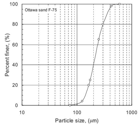
Fig. 10. Particle-size distribution for Ottawa sand
