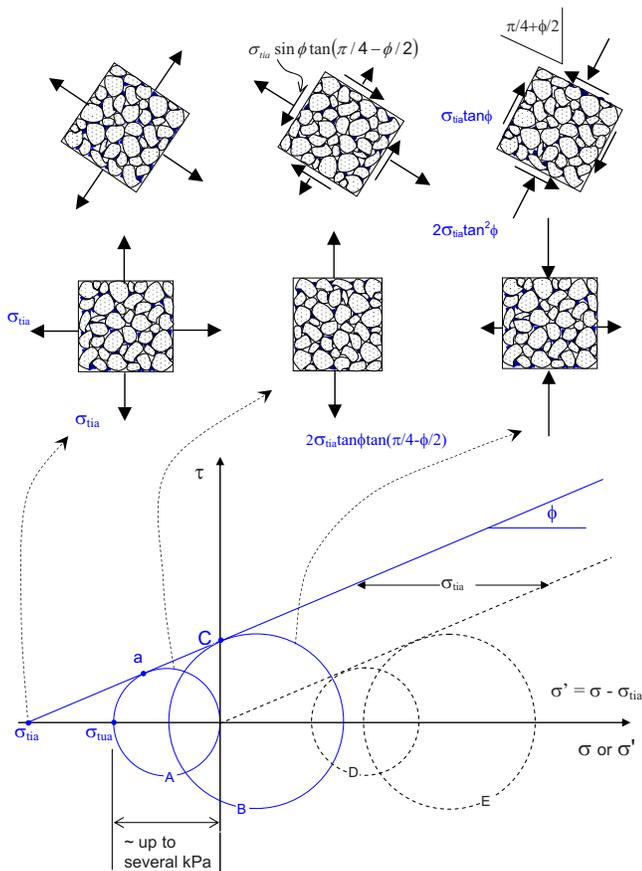
**Fig. 1.** Conceptual illustration of state of stress for isotropic tensile strength, uniaxial tensile strength, and apparent cohesion for M-C failure. Solid curve and circle are for the total stress representation whereas dashed curve and circle are for the effective stress representation.
