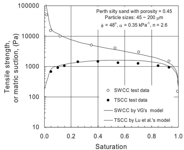
**Fig. 8.** Experimental validation of tensile strength theory for Perth silty sand: (a) particle-size distribution; (b) experimental data versus theoretical prediction
