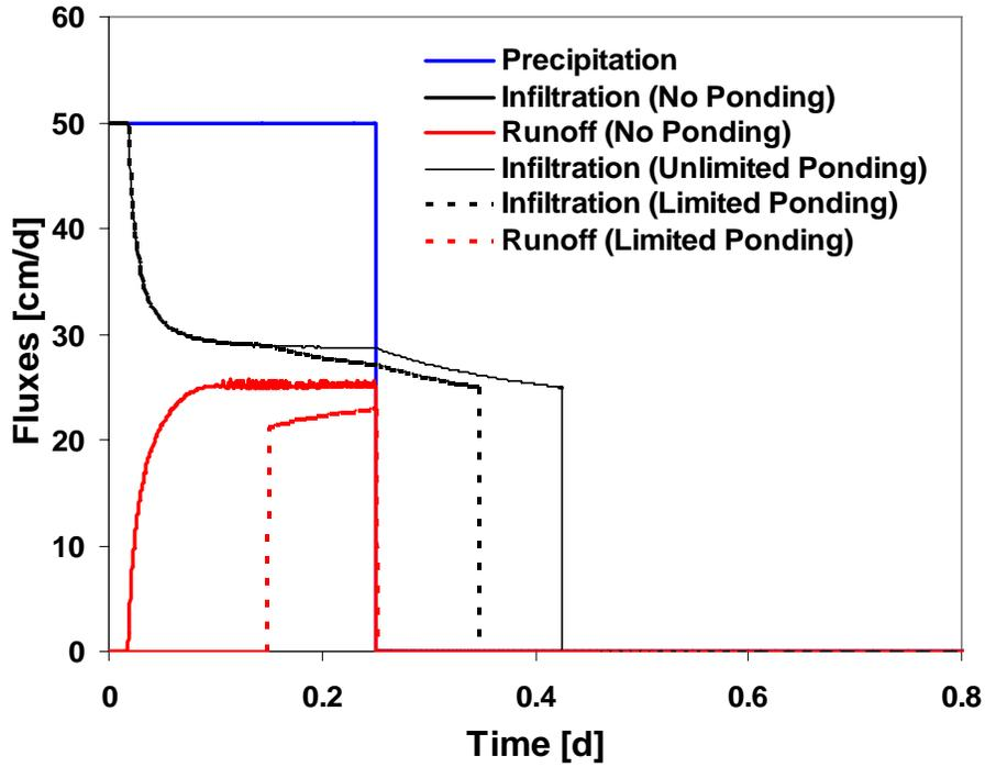
Figure 2. Infiltration fluxes and surface runoff for three scenarios of infiltration from a high-intensity rainfall event in a loamy soil with (unlimited or limited) and without surface ponding.
