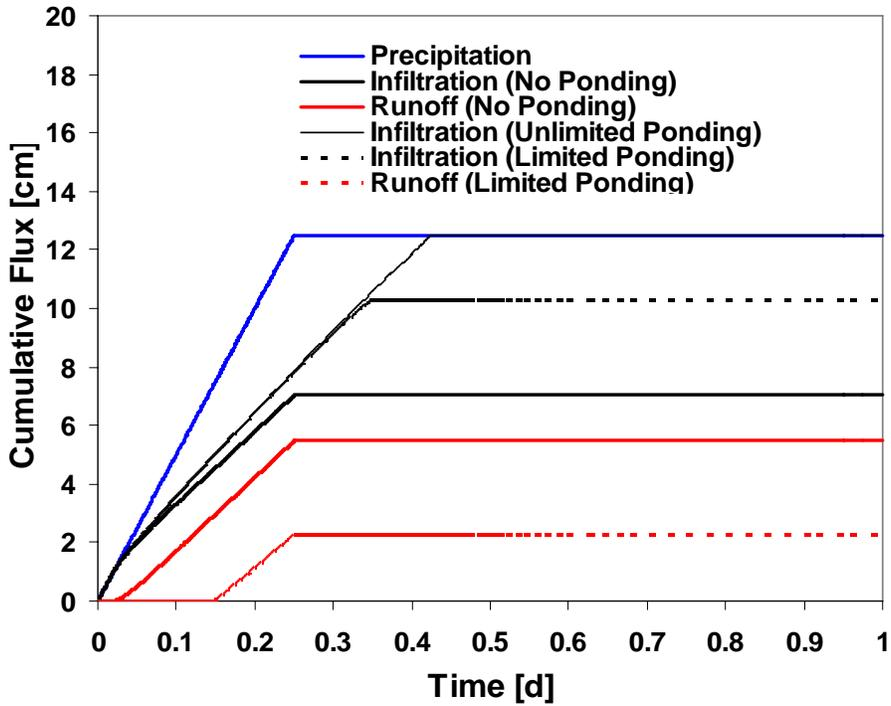
Figure 3. Infiltration fluxes and surface runoff for three scenarios of infiltration from a high-intensity rain rainfall event in a loamy soil with (unlimited or limited) and without surface ponding.
