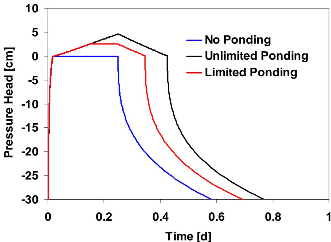
Figure 1. Pressure heads in the surface node for three scenarios of infiltration from a high-intensity rain rainfall event in a loamy soil with (unlimited or limited) and without surface ponding.
