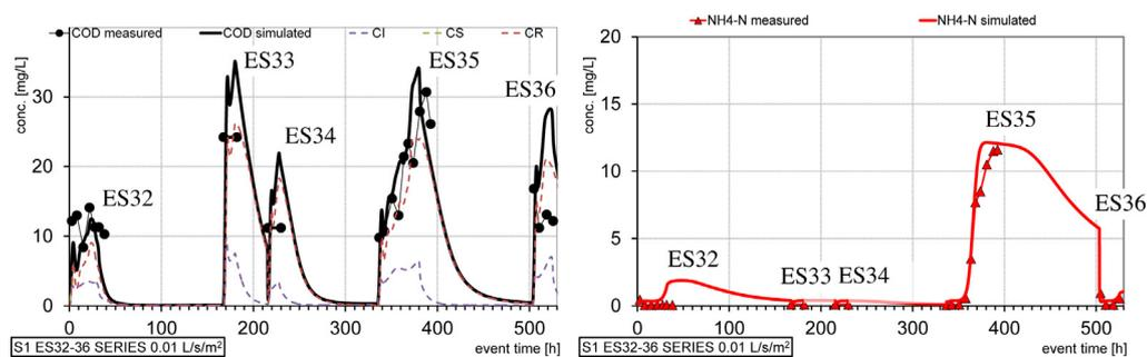
Fig. 5. Model validation with a series of five consecutive loadings, ES32–36. Simulation is continuous but measurements were made during the intra-event periods exclusively.
