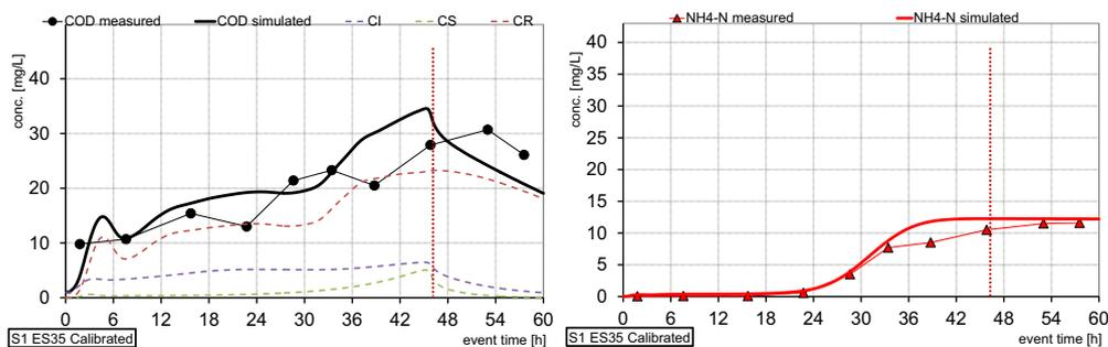
**Fig. 3.** Calibration results on COD and NH<sub>4</sub>-N. The red dotted line marks the outflow rate getting lower than the flow limitation. (For interpretation of the references to colour in this figure legend, the reader is referred to the web version of this article.)
