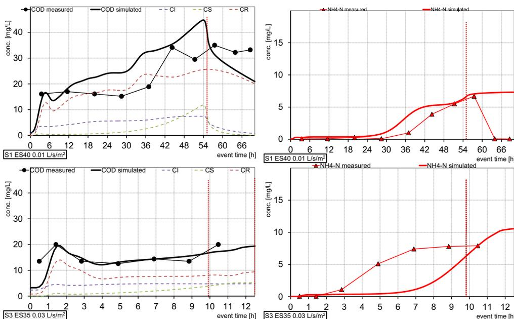
Fig. 4. Validation results from domains with different flow limitations. Top: 0.01 L/s/m<sup>2</sup>, bottom: 0.03 L/s/m<sup>2</sup>, left: COD and COD fractions, right: NH<sub>4</sub>-N.
