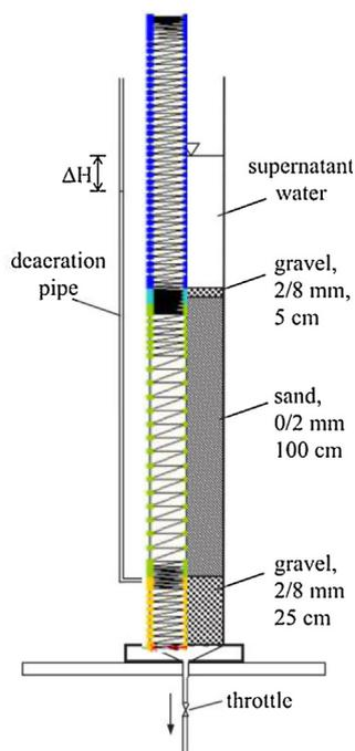
**Fig. 1.** Section draft of the physical columns (based on Meyer, 2011).  $D = 19$  cm. The left side to the symmetry axis is swapped to the left half of the finite element mesh used in the simulations.
