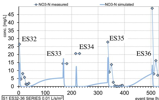
Fig. 6. Comparison of measured and simulated flush of NO<sub>3</sub>-N of five consecutive loadings, ES32–36.
