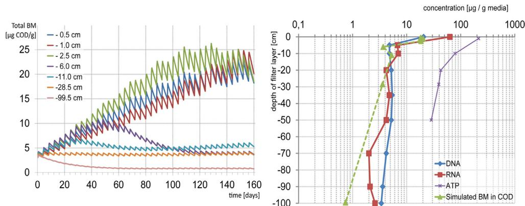
**Fig. 2.** Biomass (BM) development and vertical distribution at equilibrium. Simulated concentrations during 160 days of inoculation (left) and comparison of the final distribution at day 160 with DNA, RNA and ATP measurements (Woźniak, 2007) along the vertical profile of the filter (right). (For the colours on the left chart, the reader is referred to the web version of the article.)
