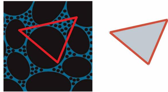
**Figure 2** | Schematic sketch of the subsurface: the simplified 'reality' (left) and the finite-element approach (right).
