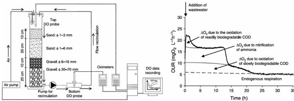
**Figure 3** | Respirometer for monitoring oxygen consumption (left) and examples for a respirogram (right) (Andreottola *et al.* 2007).
