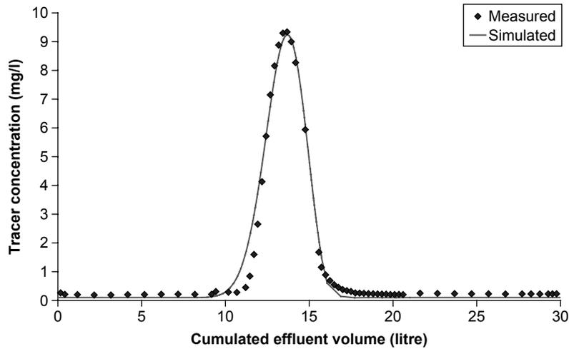
**Figure 3** Measured and simulated breakthrough curves of column 6
