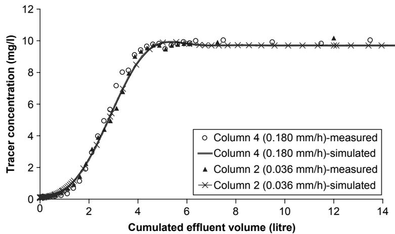
**Figure 4** Measured and simulated breakthrough curves for controlled effluent flow rate
