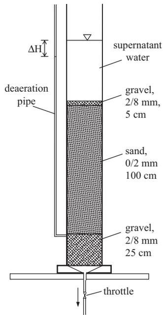
**Figure 1** Lab-scale filter column
