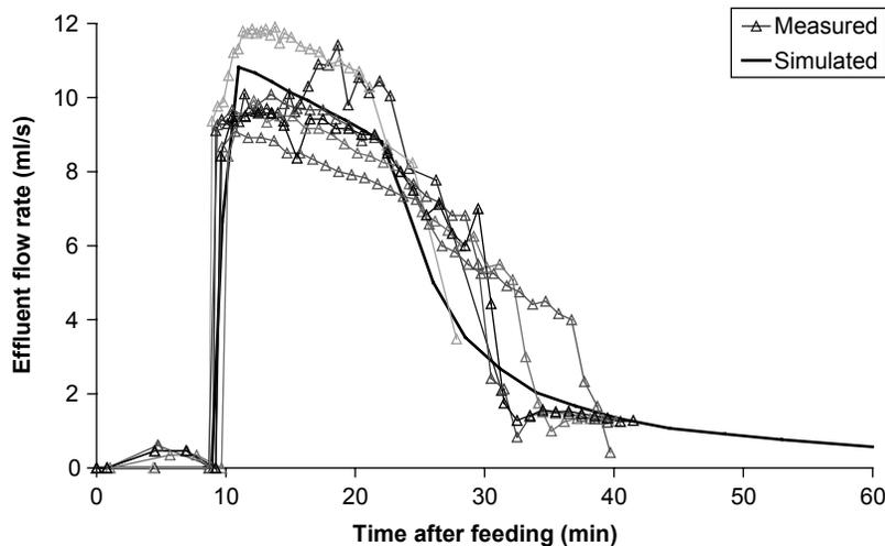
Figure 2 Measured and simulated effluent flow rate for free drainage
