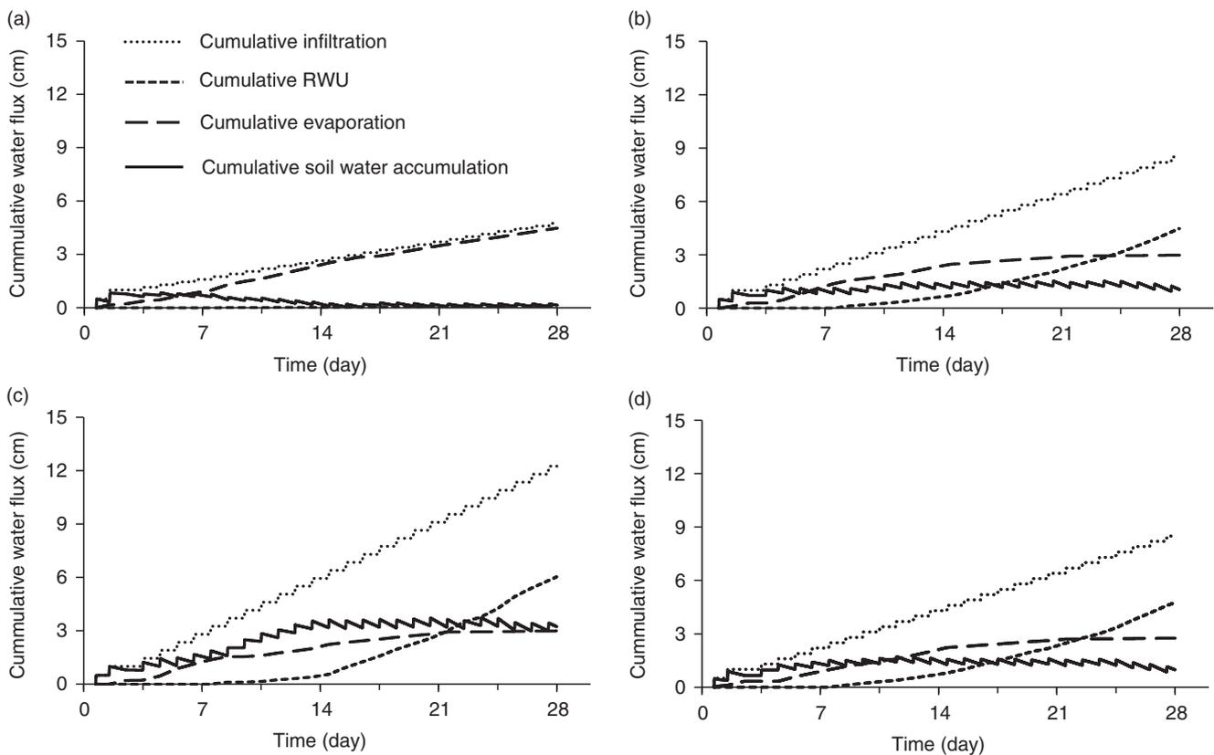
**Figure 7** Simulated cumulative infiltration, root water uptake (RWU), evaporation and soil water accumulation at different times. Results for the soil containers with a CB and irrigation rates of 0.15, 0.30 and 0.45 cm/day are shown in (a), (b) and (c), respectively. Results for the soil container without a CB and the irrigation rate of 0.30 cm/day are displayed in (d).
