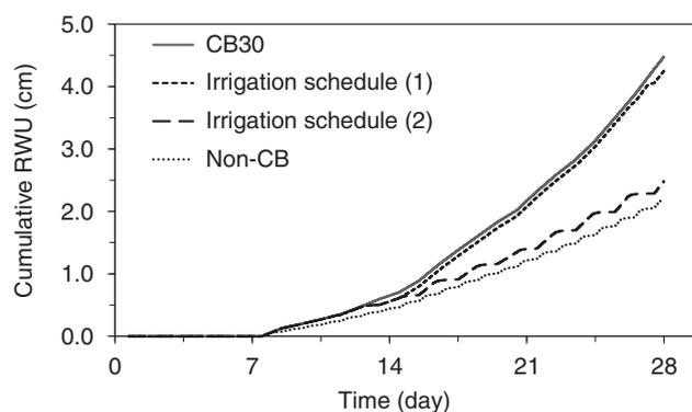
**Figure 8** Cumulative root water uptake (RWU) for different irrigation strategies based on CB30. The irrigation schedule (1) involves the soil container with a CB in which 0.30 cm of water was applied every other day during the first stage of plant growth (from day 4 to day 14). The irrigation schedule (2) involves the soil container with a CB where 0.30 cm of water was applied every 2 days during the entire growing period. The non-CB scenario represents the soil profile without a CB.
