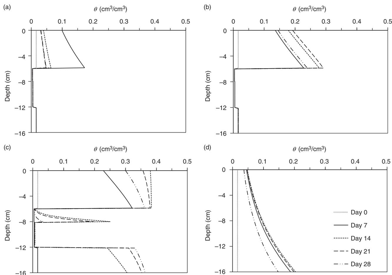
**Figure 6** Simulated volumetric soil water contents at different times. Results for the soil containers with the CB and irrigation rates of 0.15, 0.30 and 0.45 cm/day are shown in (a), (b) and (c), respectively. Results for the soil container without a CB and the irrigation rate of 0.30 cm/day are in (d).
