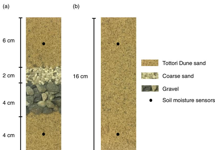
**Figure 1** The soil profiles with (a) and without (b) a capillary barrier (CB) layer in the cultivation experiment (Miyake *et al.*, 2015). [Colour figure can be viewed at [wileyonlinelibrary.com](http://wileyonlinelibrary.com)]
