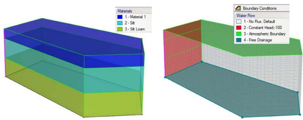
Fig. 6. The transport domain showing the assumed materials (left) and boundary conditions (right) as specified on Geometric Objects.
