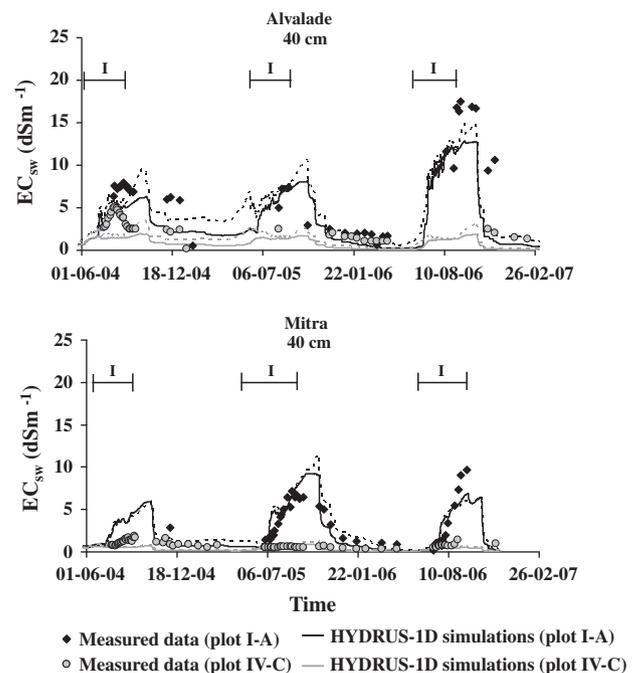
**Fig. 5.** Measured and simulated soil solution electrical conductivities at a 40-cm depth in Alvalade (top) and Mitra (bottom). Symbol I denotes the irrigation periods. Full lines represent the results of the major ion chemistry module (the UNSATCHEM module). Dashed lines represent the results obtained with the standard HYDRUS solute transport module.
