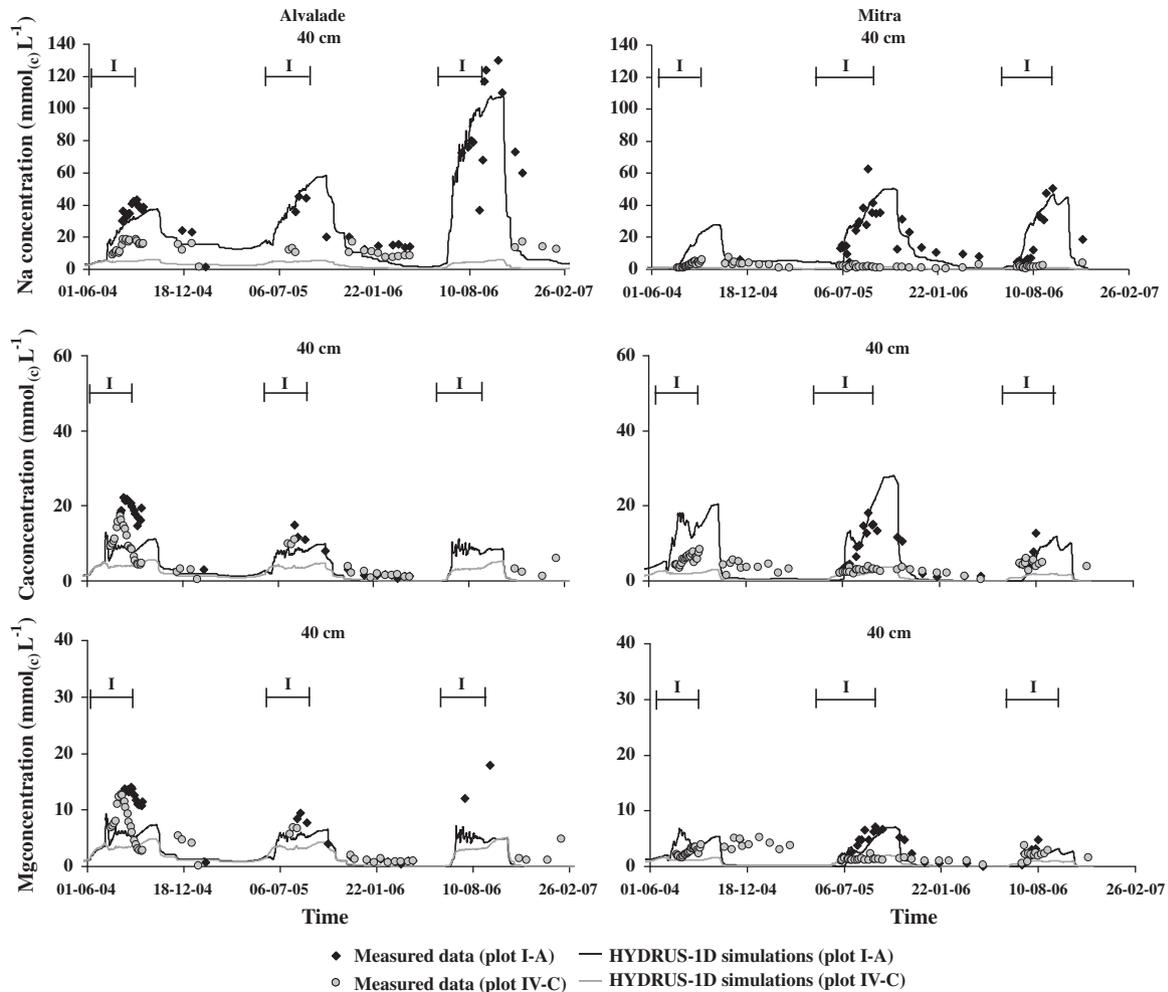
**Fig. 6.** Measured and simulated soluble sodium (top), calcium (middle), and magnesium (bottom) concentrations at a 40-cm depth in Alvalade (left) and Mitra (right). Symbol I denotes the irrigation periods.
