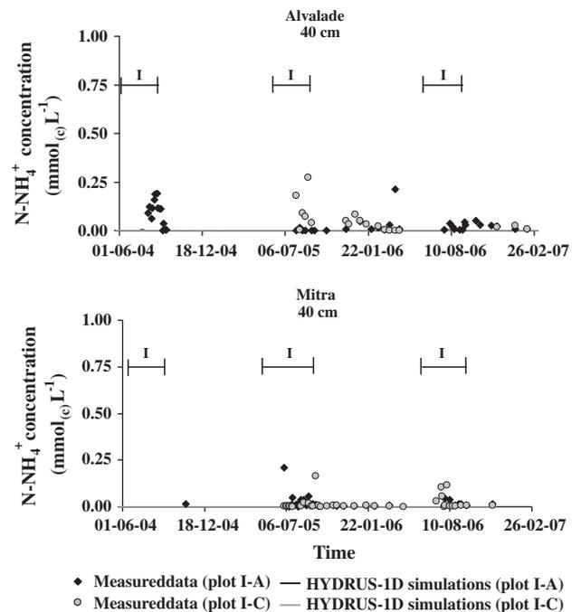
**Fig. 8.** Measured and simulated ammonium concentrations at a 40-cm depth in the experimental plots of group I in Alvalade (top) and Mitra (bottom). Symbol I denotes the irrigation periods.
