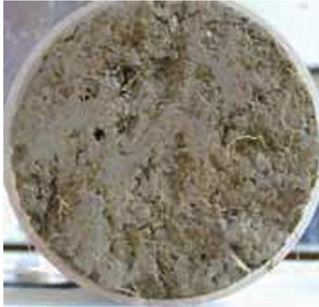
Fig. 4. Photo of the soil structure at the bottom of column I.
