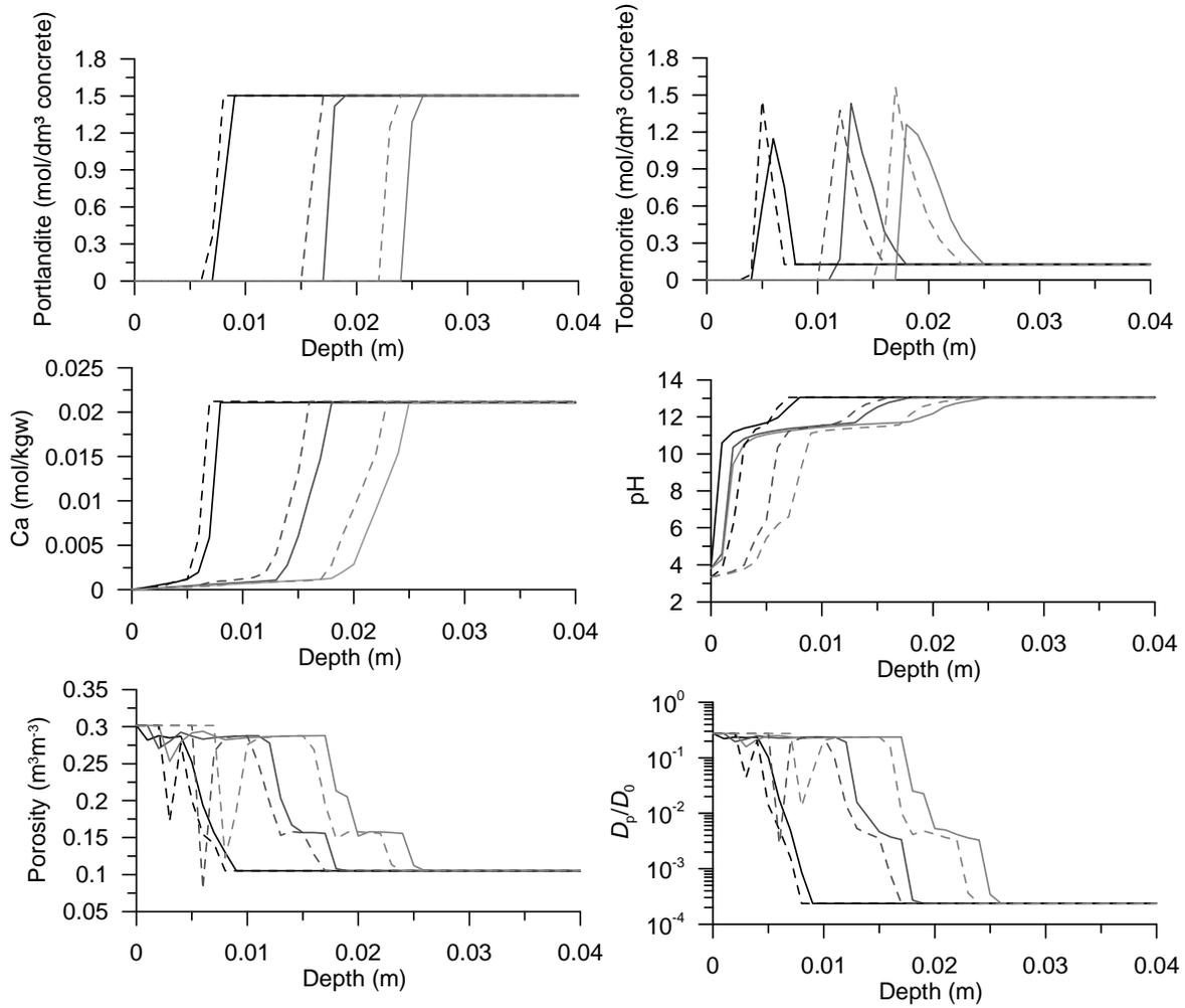
Figure 1. Profiles of different geochemical state variables in concrete after 50 (black), 150 (dark grey) and 300 (light grey) years during diffusive leaching with rain water (full line) or soil water (dashed line).
