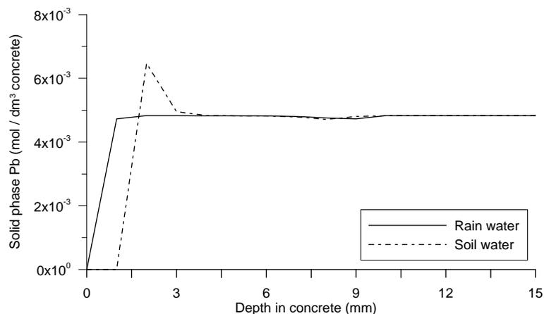
Figure 2. Solid phase Pb profiles after 20 years leaching of cementitious waste during diffusive transport conditions.
