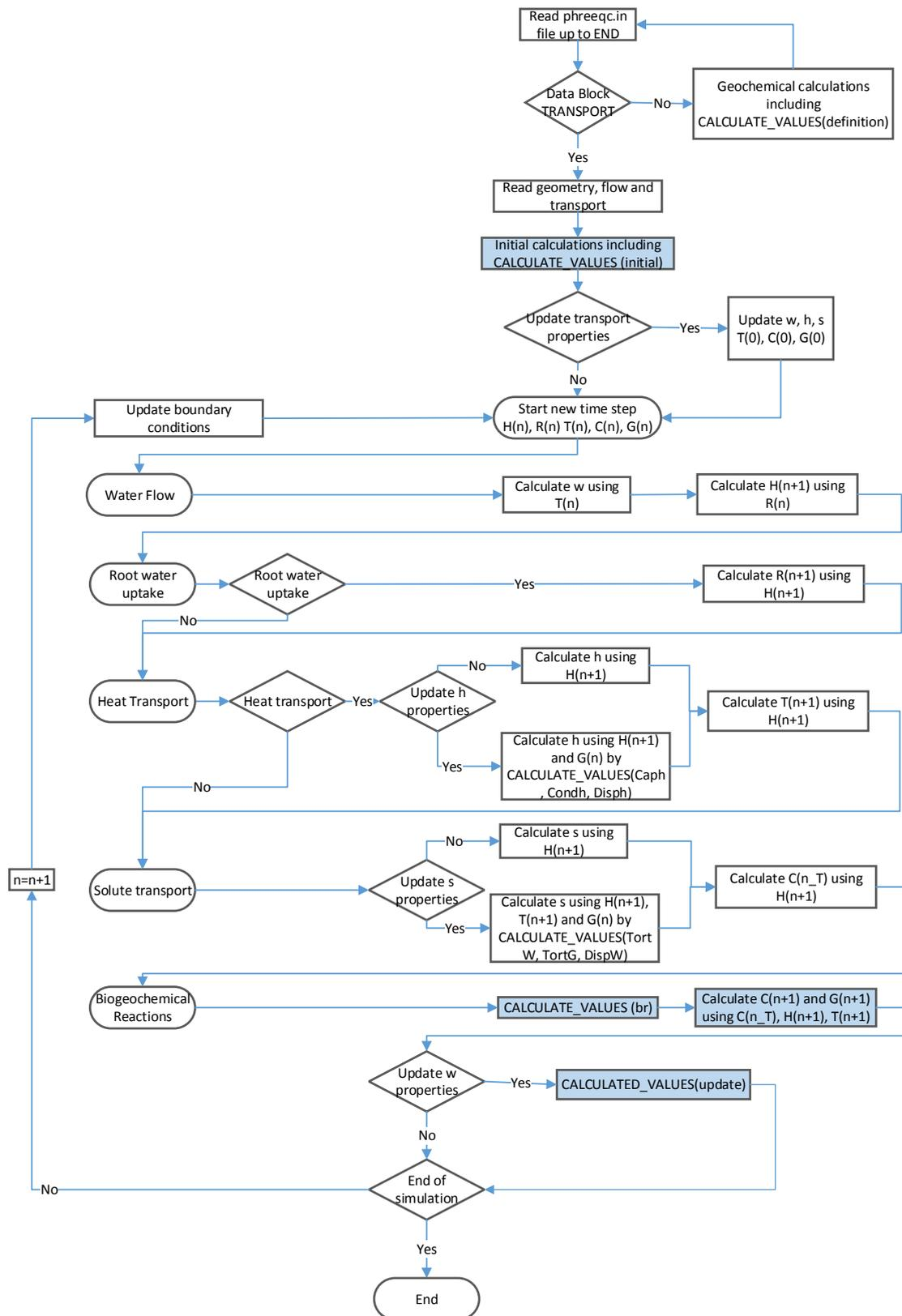
**Fig. 2.** Flow chart of HPx. The letters w, h, and s indicate parameters for water flow, heat transport, and solute transport, respectively. The variables H, R, T, C, and G indicate state variables for water flow, root water uptake, heat transport, solute transport, and biogeochemical processes, respectively. The boxes with blue background are steps run in parallel using OpenMP. CALCULATED\_VALUE(type) indicates the execution of scripts labeled with type.
