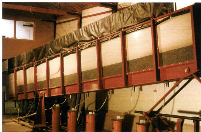
**Fig. 1.** A front view of the filled 10-m tipping trough (dark brown material = capillary block, light-colored material = capillary layer, and collection sump in the left-most segment). A dye tracer experiment with a red tracer is depicted on the left side. The irrigation system is inside the black box on the top of the tipping trough. Photo: Institute of Soil Science, University of Hamburg.
