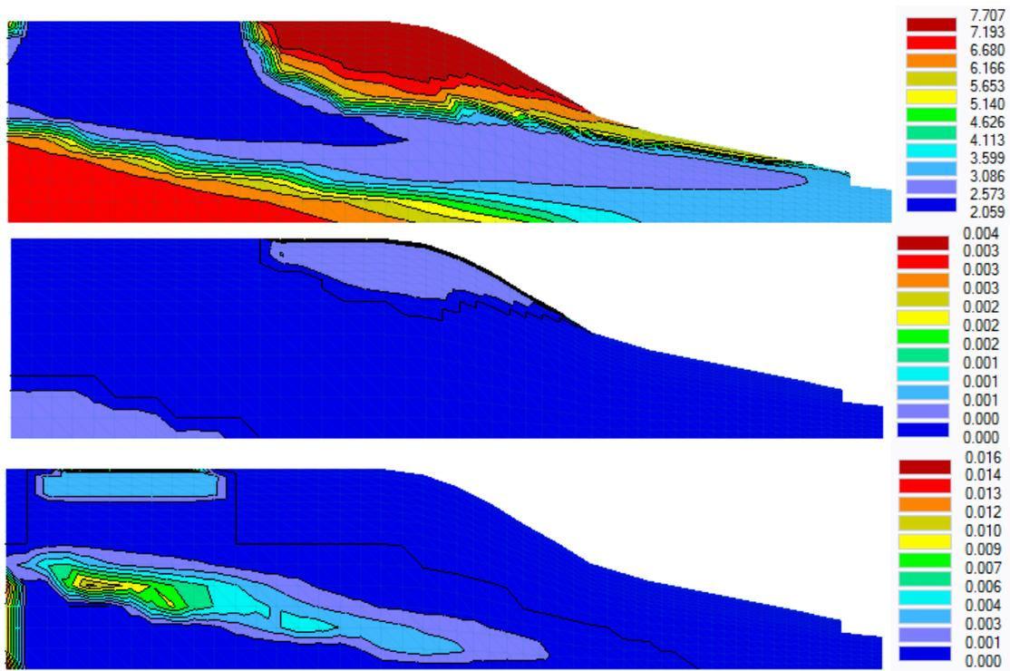
Figure 28. pH (top), calcite (mol/L) (middle), and gypsum (mol/L) (bottom) profiles after 1000 d for the Tailing Pile Leaching example.
