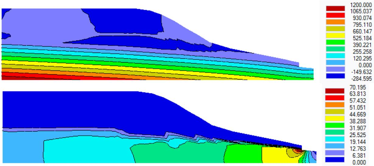
Figure 26. The steady-state pressure head (cm) (top) and flux (cm/d) (bottom) profiles for the Tailing Pile Leaching example.
