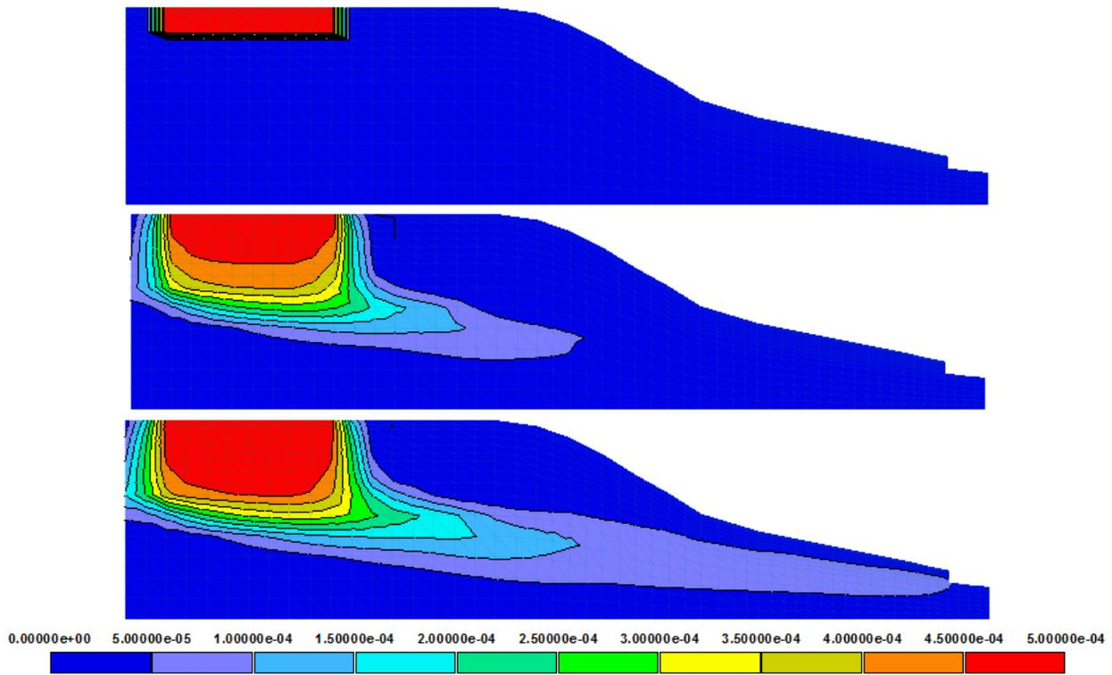
Figure 27. Uranium concentration profiles at time 0 (top), 250 (middle), and 500 (bottom) d for Tailing Pile Leaching example.
