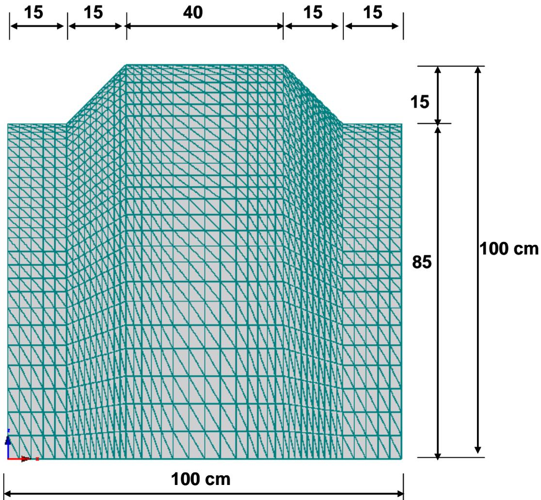
Figure 20. Schematic representation and finite element mesh of the flow domain for the furrow irrigation system for example 4.
