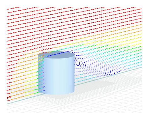
**1.2.** Very tall cylinder. Kármán eddies can be simulated, but it requires a very fine mesh around the cylinder and in the space behind it. This mesh should have at least 10 - 100 million cells, and calculating the transient flow with the Karman vortex street would take several days on a high-end PC.
