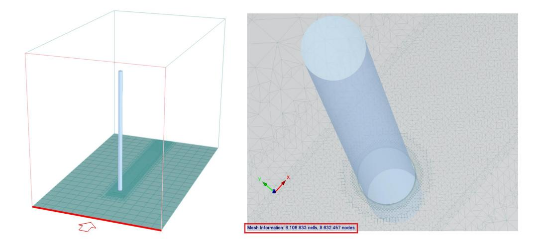
**1.3.** Pseudo-2D simulation. It is well known that Kármán eddies can be easily simulated in 2D. In 3D we can do a similar simulation using a wind tunnel with a very low height (manually set) and a special 3D mesh for this pseudo-2D case.
