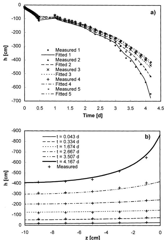
**Fig. 6. Measured and fitted tensiometer readings for Experiment I as a function of (a) time and (b) depth.**
