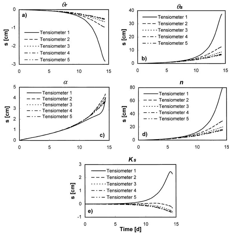
Fig. 2. Sensitivity of the pressure head  $h$  to parameters (a) residual soil water content,  $\theta_r$ , (b) saturated water content,  $\theta_s$ , (c)  $\alpha$ , (d)  $n$ , and (e) saturated hydraulic conductivity,  $K_s$ , as a function of time for a silty soil assuming a one-step evaporation experiment.
