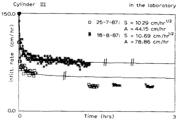
Fig. 7. Courses of the infiltration rate for two series of recurrent measurements taken on cylinder III in the laboratory at various days with different initial moisture contents. Values of steady-state infiltration rates of the first series (marked as  $\square$ ) are 57.98 and 37.73  $\text{cm h}^{-1}$ . Values of steady-state infiltration rates of the second series (marked as  $*$ ) are 72.24, 40.06 and 37.99  $\text{cm h}^{-1}$ .
