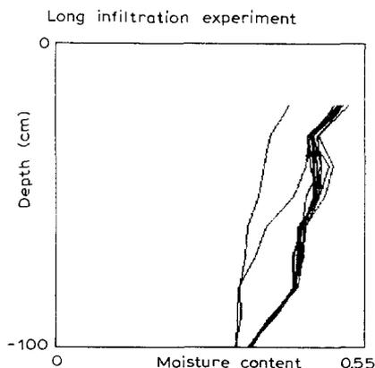
Fig. 2. Soil moisture profiles measured during the long infiltration experiment inside the inner cylinder by the Troxler neutron probe. The first curve is measured at the start, the other curves are measured at times (h. min) 0.10, 0.30, 0.45, 1.00, 1.15, 1.30, 2.30, 3.15, 4.30 and 9.00 after the start.
