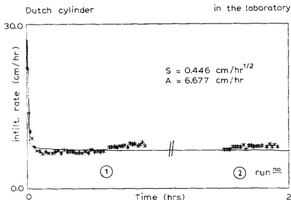
Fig. 8. Courses of the infiltration rate for two recurrent measurements on Dutch cylinder in the laboratory. Values of steady-state infiltration rates are  $8.16$  and  $7.81 \text{ cm h}^{-1}$ . This series had four recurrent measurements in total; the further two, which are not plotted, showed values of steady-state infiltration rates of  $7.49$  and  $7.49 \text{ cm h}^{-1}$ .
