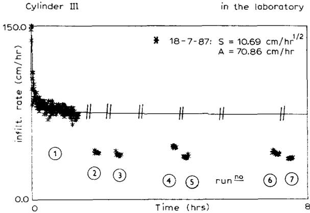
Fig. 6. Courses of the infiltration rate for seven recurrent measurements on cylinder III in the laboratory. Values of steady-state infiltration rates are 72.24, 40.06, 37.99, 44.96, 35.54, 39.70 and 34.70  $\text{cm h}^{-1}$ , respectively.
