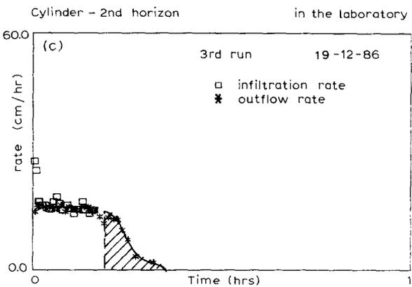
Fig. 5. Courses of the infiltration and outflow rates measured in consecutive days in the laboratory for the cylinder taken from the 2nd horizon. Values of tensiometer reading are shown in Table 4 together with values of steady-state infiltration rates and information about outflow. Note changes in post-infiltration outflow volume (hatched areas)
