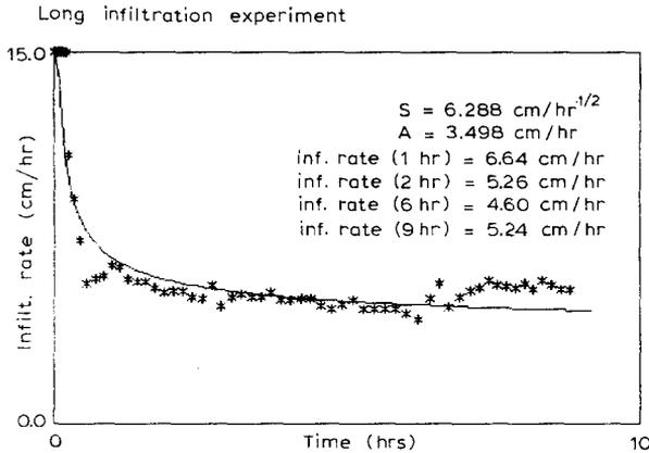
Fig. 1. The course of the long infiltration experiment measured in the field and compared with infiltration theory.
