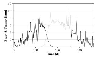
**Figure 4** Mean daily values of potential evaporation (black line) and potential transpiration (grey line) during the simulation period.
