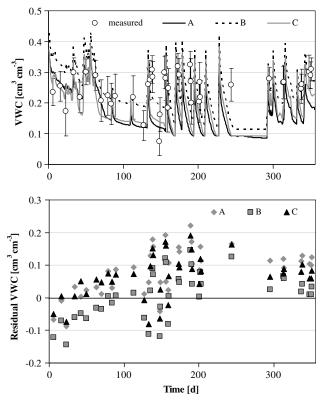
Figure 5 Measured and simulated volumetric water contents (VWC) (cm<sup>3</sup> cm<sup>-3</sup>) averaged over the top soil layer at mean daily measurement times (top). Error bars represent one standard deviation resulting from spatial averaging. Residual (measured minus modeled) volumetric water contents (bottom). Cases A, B, and C are the same as in Fig. 3.
