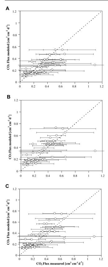
**Figure 8** A comparison of measured and simulated  $CO_2$  fluxes (cm<sup>3</sup> cm<sup>-2</sup> d<sup>-1</sup>). The dotted line represents 1:1 line. Error bars at measured values represent one standard deviation resulting from spatial averaging. Cases A, B, and C are the same as in Fig. 3.
