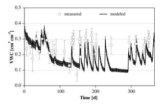
**Figure 9** Volumetric water contents (VWC) (cm<sup>3</sup> cm<sup>-3</sup>) calculated using varied soil hydraulic properties (listed in Table 4). Error ranges (black shade) associated with simulated VWCs represent  $\sigma_{\theta_w}$ .
