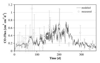
**Figure 10** Simulated and measured CO<sub>2</sub> fluxes calculated using varied soil hydraulic properties (listed in Table 4). Error ranges (black shade) of simulated CO<sub>2</sub> fluxes represent  $\sigma_{q_r}$ .
