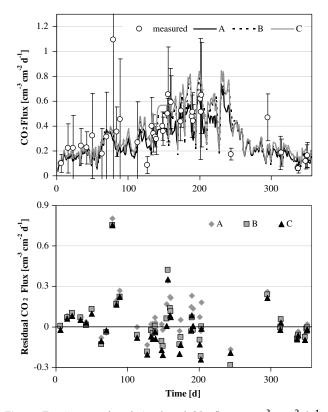
**Figure 7** Measured and simulated  $CO_2$  fluxes (cm<sup>3</sup> cm<sup>-2</sup> d<sup>-1</sup>) at mean daily measurement times (top). Error bars represent one standard deviation resulting from spatial averaging. Residual (measured minus modeled)  $CO_2$  fluxes (bottom). Cases A, B, and C are the same as in Fig. 3.
