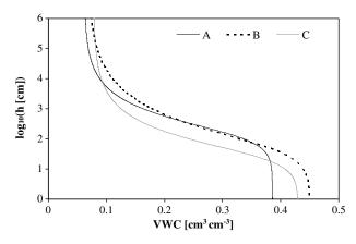
**Figure 3** Retention curves corresponding to soil hydraulic parameters presented in Table 2. These parameters were obtained using (A) neural network predictions with Rosetta (Schaap et al., 2001), (B) average parameters for the silt loam textural class (Carsel and Parrish, 1988), and (C) average parameters for the loam textural class (Carsel and Parrish, 1988). VWC – volumetric water content.
