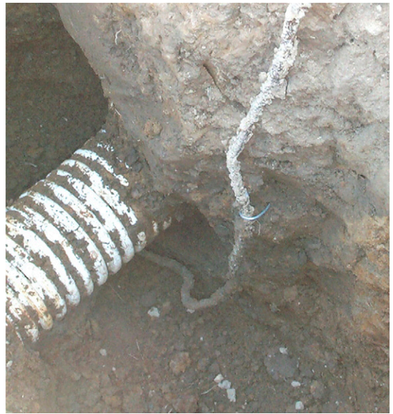
FIG. 1. A photograph of a natural, directly connected macropore in the field preserved with polymer resin, demonstrating the connection between a macropore and a subsurface drain (courtesy of Martin Shipitalo, USDA-ARS, Coshocton, OH).
