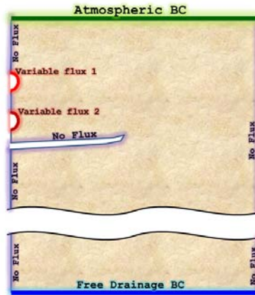
Figure 3. The transport domain with applied boundary conditions.
