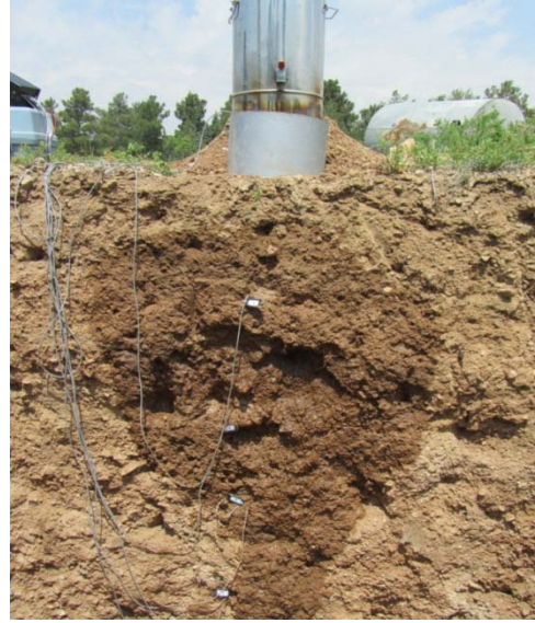
Figure 1b. Location of four thermal sensors.
