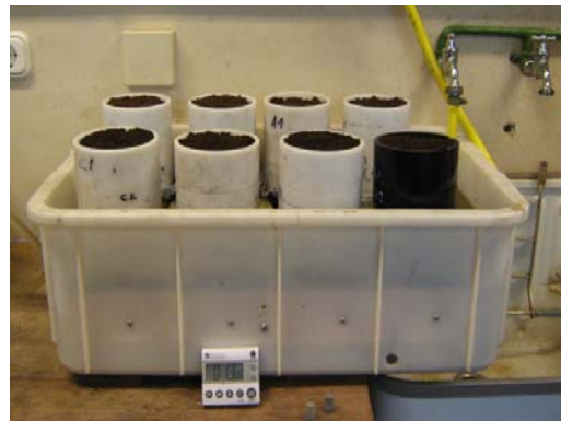
Figure 3. Experimental containers with 10 cm inner diameter and 15 cm height.
