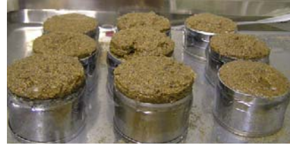
Figure 8 Expanded volume by swelling.
